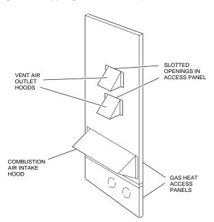
FIGURE 8 - VENT AND COMBUSTION AIR HOOD
